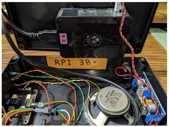
Plug in the RPI when ready to test, but leave the final screw-tight mounting in project box as one of final steps when everything works on the network.
